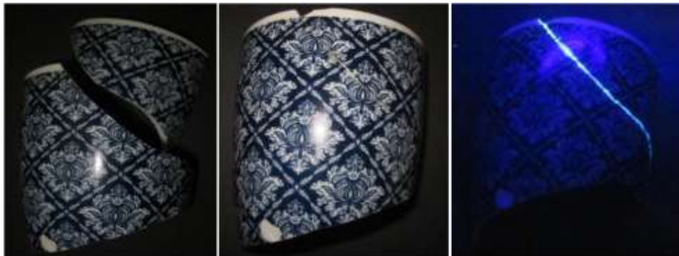
Figure depicting a broken design, joined by the adhesive and the visibility of the fractured joint observed under the UV light (365 nm)
