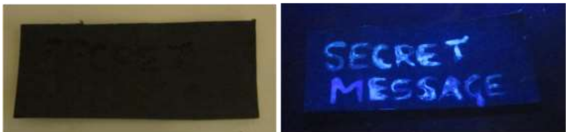
Figure depicting the visibility of the words written by the adhesive under UV light (365 nm), which are invisible under normal light
